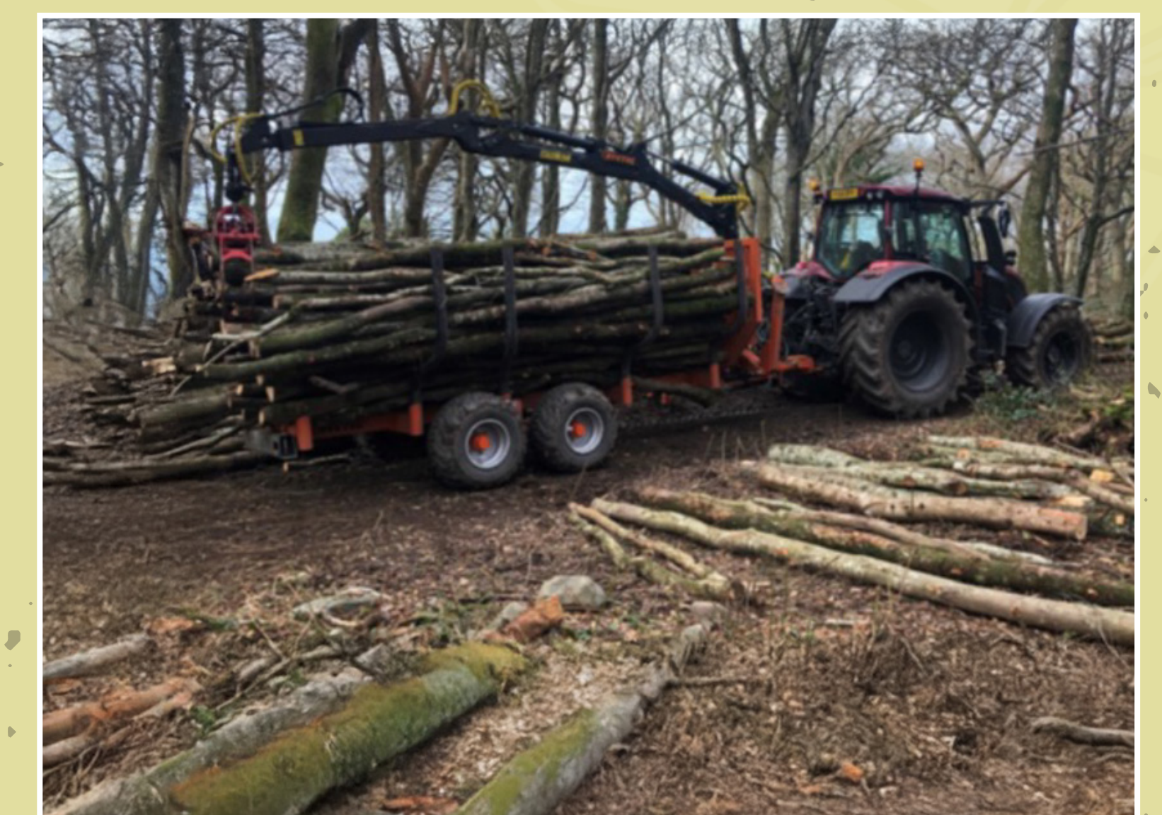
Figure 3 and 4. Timber extraction from track side undertaken with horses as high ecological interest at the site favoured a low impact method, before extraction via tractor and forwarding trailer to stacking area.
